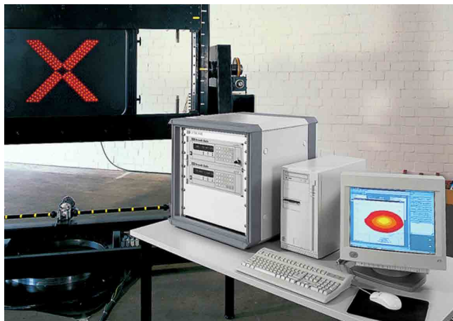
Client specific Goniophotometer design - one of our strengths. Goniophotometer for traffic signs and lights of large dimension and weight
