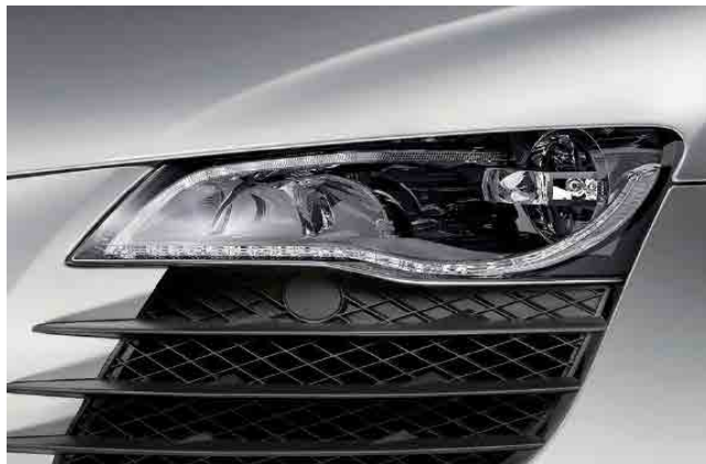
Full LED headlamp; PWM LED sources are a challenge we found a solution for DSP 10
