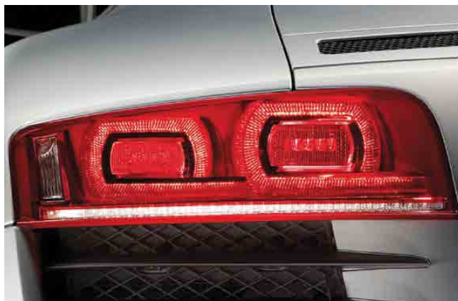
Full LED rear lamp with pulse width modulation and short duty cycles
