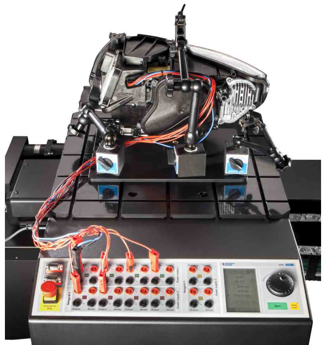
RecoCAN-L multiplexer and control unit with 10 channels for three power supplies simultaneously operated, touch screen with extended operating functions including a direct selection of power supply channel and manual positioning options in fast and fine adjustment mode. Optional connection of AFS data interface and temperature measurement of LED modules.
