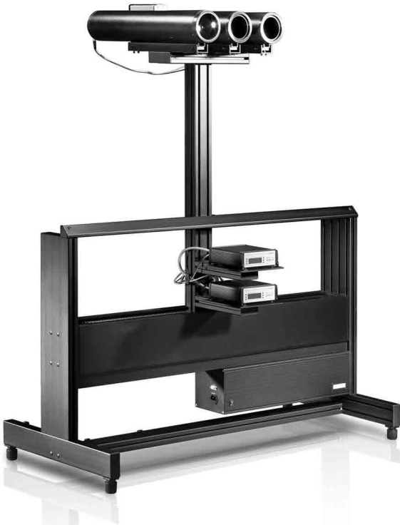
Automatic photometer tube positioning unit PPE10 with LM 20 and 3.162 m detector for luminous intensity measurement
