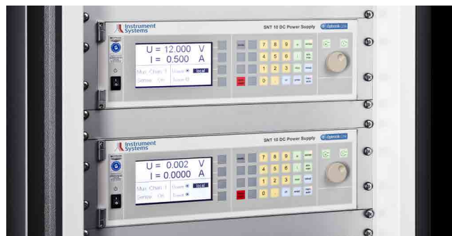
SNT 10 - System power supply fully integrated by CAN-Bus supporting 4 channels power and sense each
