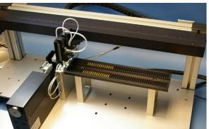
CYC801 Cyclic Tester: to measure tensile fatigue properties of fibre samples subjected to repeated strain, force or stress.
