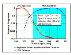
Fig. 1. Model 3D Spectral Response
