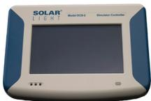
**Sophisticated Automatic Dose Controllers** measure the spectral response following the Erythema Action Spectrum and UVA Spectrum to allow accurate dose control when measuring SPF values. The 7-inch (17.8 cm) touch sensitive screen allows the user to follow intuitive menus and makes it quick and easy to set control parameters.
